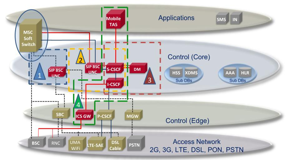
Note: The MSC is replaced in stage 4 by Mobile Telephone Application Server (TAS) and IMS Call Server Access Gate Way (ICS GW)
